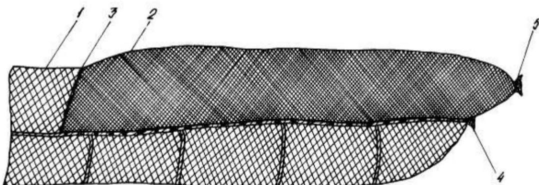
**Figure 3.8.2.** Codend bag scheme: 1 - main bag 2 - apron; 3 - connector, 4 - the main bag 5 - the trailer outer bag connection.
