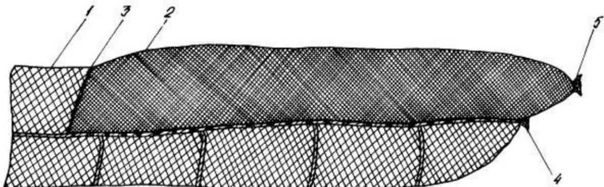
Figure 3.8. Codend bag scheme: 1 - main bag 2 - apron; 3 - connector, 4 - the main bag 5 - the trailer outer bag connection.
